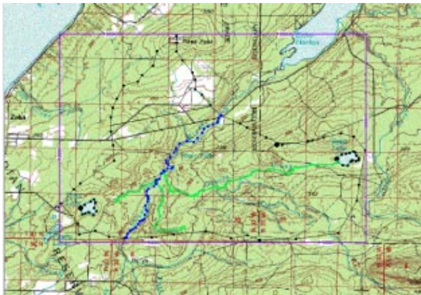
Figure 6: Watershed boundaries with the delineated Silver River (blue), drains (green) and constant head lakes (black).
